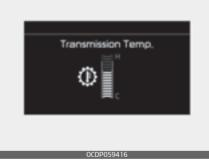
This mode displays the transmission temperature.
