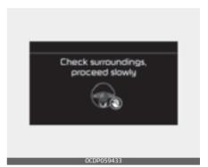
• The above message will appear if the shift lever is in D (Drive) or R (Reverse) according to the distance of the front and rear object from the sensor.
