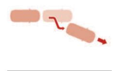
When driving in stop-and-go traffic, and a stopped vehicle in front of you merges out of the lane, FCA system may not immediately detect the
