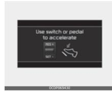
While Smart Cruise Control system is in operation, your vehicle stops behind the vehicle in front when it stops. The message is displayed on the cluster within 3 seconds after the stop and the system will be in the standby position. If the driver does not take action for a certain period of time after the vehicle in front departs, the message is displayed on the cluster.
