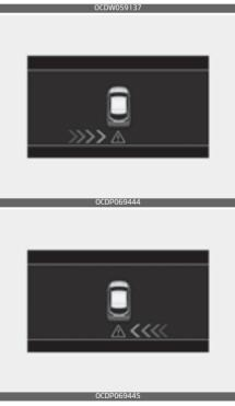
If the vehicle detected by the sensors approaches from the rear left/ right side of your vehicle, the warning chime will sound, the warning light on the outside rearview mirror will blink and a message will appear on the LCD display. If the rear view monitor system is in activation, a message will also appear on the infotainment system screen.
