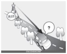
Flutter/Static – Weak FM signals or large obstructions between the transmitter and your radio can disturb the signal causing static or fluttering noises to occur. Reducing the treble level may lessen this effect until the disturbance clears.
