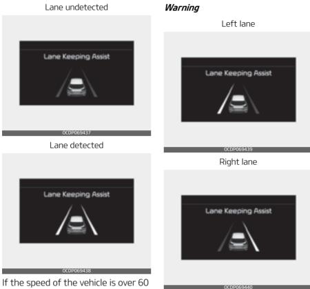
If the speed of the vehicle is over 60 km/h (37 mph) and the system detects lane markers, the color changes from gray to white.
