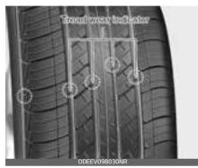
This shows there is less than 1.6 mm (1/16 in.) of tread left on the tire. Replace the tire when this happens.
