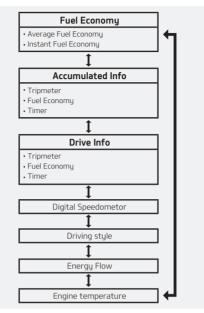
To change the trip mode, scroll the MOVE scroll switch ( $\land$  /  $\checkmark$ ) in the trip computer mode.
