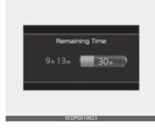
It is also displayed, when the driver's door is opened with charging in progress. When scheduled charging is set, the estimated charging time is displayed as "--".
