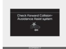
When FCA is not working properly, FCA warning light (Solution) will illuminate and the warning message will appear for a few seconds. After the message disappears, the master warning light (A) will illuminate. In this case, have the vehicle inspected by a professional workshop. Kia recommends to visit an authorized Kia dealer/service partner.
