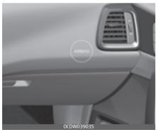
Your vehicle is equipped with a Supplemental Restraint (Air Bag) System and lap/shoulder belts at both the driver and passenger seating positions. The indications of the system's presence are the letters "AIRBAG" engraved on the air bag pad cover in the steering wheel and the passenger's side front panel pad above the glove box.
