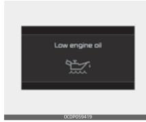
This warning message is displayed when the engine oil level should be checked.
