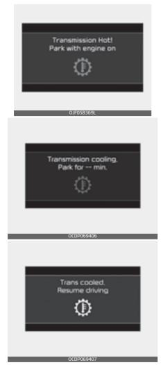
If the vehicle continues to be driven and the clutch temperatures reach the maximum temperature limit, the "Transmission Hot! Park with engine on" warning will be displayed. When this occurs the clutch is disabled until the clutch cools to normal temperatures.
