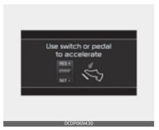
Use switch or pedal to accelerate
