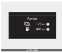
The range is the estimated distance the vehicle can be driven with the remaining high-voltage (hybrid) battery (1, Electric) and fuel in the fuel tank (2, Gasoline).
