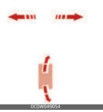
• Push the sunroof control lever backward to the first detent position.
