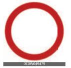
The symbol is displayed on the instrument cluster and the navigation, when ISLW does not have any reliable speed limit information.
