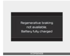
If SOC (State of High voltage battery Charge) is high, it is not possible to enable Regen B mode. Use the function again after normal driving.
