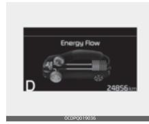
The hybrid system informs the driver about its energy flow in various operating modes. While driving, the current energy flow is specified in 11 modes.
