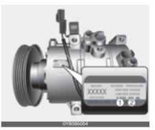
A compressor label informs you the type of compressor your vehicle is equipped with such as model, supplier part number, production number, refrigerant (1) and refrigerant oil (2).
