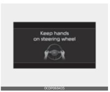
If you keep your hands off the wheel while driving with LFA system assisting the steering, the handsoff warning will be triggered.
