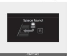
While driving forward to search for a parking space, the above message will appear with a beep sound if the search is complete. Stop the vehicle and shift to the R (Reverse) position.
