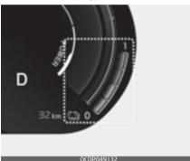
This gauge indicates the remaining hybrid battery power. If the SOC is near the "L (Low) or O" level, the vehicle automatically operates the engine to charge the battery. However, if the Service Indicator (A) and Malfunction Indicator Lamp (MIL) (X) turn on when the SOC gauge is near the "L (Low) or O" level, have the vehicle checked by a professional workshop. Kia recom-
