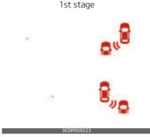
If a vehicle is detected within the boundary of the system, a warning light will illuminate on the outside rear view mirror.
