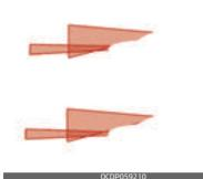
If the vehicle in front of you has cargo that extends rearward from the cab, or when the vehicle in front of you has higher ground clearance, additional special attention is required. FCA system may not be able to detect the cargo extending from the vehicle. In these instances, you must maintain a safe braking distance from the rearmost object, and if necessary, depress the brake pedal to reduce your driving speed in order to maintain distance.
