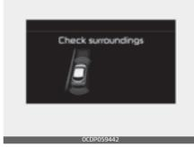
Parking Assist checks the front and rear space to exit the vehicle from the parking space.
