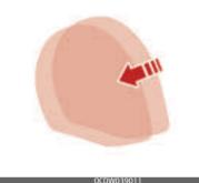
The headrest may be adjusted forward to 4 different positions by pulling the headrest forward to the desired detent.
