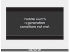
If the motor and battery is in high/low temperature status or if there is a malfunction on battery and transmission, the warning message will be displayed.  If the vehicle entering the Regen B mode during the activation of ABS/Cruise Control/Smart Cruise Control, the warning message will be displayed.
