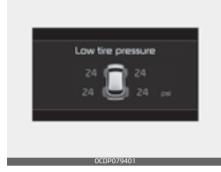
When the tire pressure monitoring system warning indicators are illuminated and warning massage displayed on the cluster LCD display, one or more of your tires is significantly under-inflated. The low tire pressure position telltale light will indicate which tire is significantly under-inflated by illuminating the corresponding position light.
