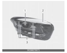
If the Low/High beam lamp(1), Front turn signal lamp(2), Day time running lamp/Position lamp(3) does not operate, have your vehicle checked by a professional workshop.
