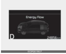
The mode means the vehicle is stopped. (There is no energy flow.)
