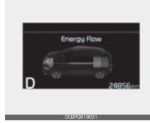
Vehicle is stopped with the Engine charging the hybrid battery.
