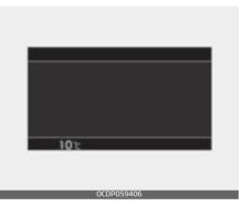
This gauge indicates the current outside air temperatures by 1°C (1°F).
