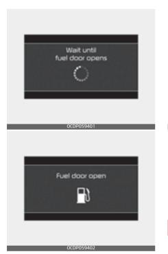
Wait until the fuel tank is depressurized. The message is displayed when the fuel filler door opens after the fuel tank is depressurized.
