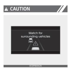
If the vehicle ahead (vehicle speed: less than 30 km/h) disappears to the next lane, the warning chime will sound and a message will appear. Adjust your vehicle speed for vehicles or objects that can suddenly appear in front of you by depressing the brake pedal according to the road condition ahead and driving condition.
