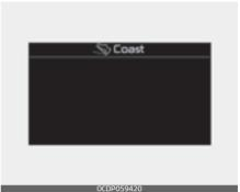
A chime will sound and the coasting guide indicator will blink four times to inform the driver when to take the foot off the accelerator by anticipating a decelerating event\* based on the analysis of driving routes and road conditions stored in the navigation system. It encourages the driver to remove the foot from the pedal and allow coasting down the road with EV motor only. This helps preventing unnecessary fuel consumption and increases fuel efficiency.
