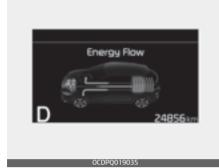
The vehicle is being slowed down by engine compression and regenerative braking. The hybrid battery is being charged by regenerative braking.
